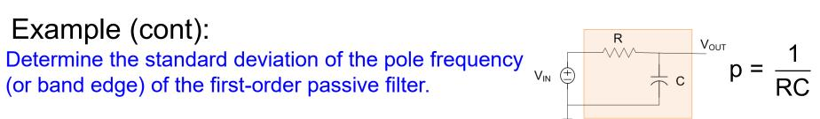
$$p = \frac{1}{\left(R_{NOM} + R_{RAN}\right)\left(C_{NOM} + C_{RAN}\right)} = \left(\frac{1}{R_{NOM}C_{NOM}}\right) \left(\frac{1}{\left[1 + \frac{R_{RAN}}{R_{NOM}}\right]\left[1 + \frac{C_{RAN}}{C_{NOM}}\right]}\right)$$
